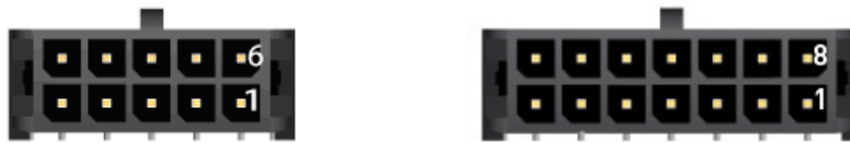
Figure 2: Pinning of the RS232 connector on a 7" device (left) and on a 5" device (right)
