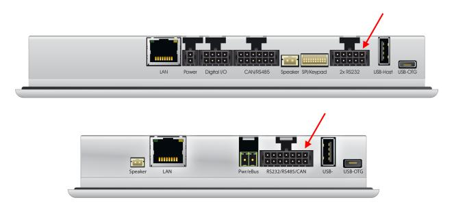
Figure 1: Location of the RS232 connector on a 7" device (upper) and on a 5" device (lower)
