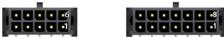
Figure 2: Pinning of the RS232 connector on a 7" device (left) and on a 5" device (right)
