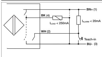
The PNP- or NPN-load will automatically be detected.
