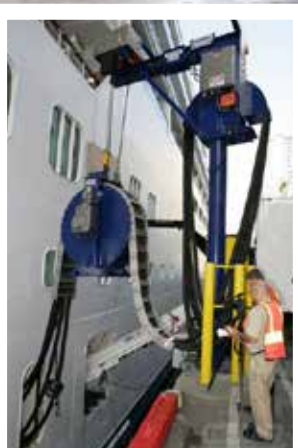
Photos feature cable on Cochran Marine's Cable Positioning Device, used to serve shore power
