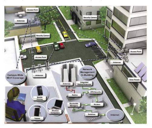
With a standard in-building DAS, the cellular source, such as a wireless base station, provides the wireless signal to the building through an antenna or wired land-line connection. In the building itself, the DAS consists of headend equipment, bi-directional amplifiers, fiber distribution remote units, and in-building antenna access points - all of which may be connected through Carol's DBRF Flexible Low Loss Coaxial Cables and General Cable's NextGen® Brand fiber optic cables.
