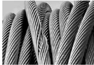
Figure 7 – T-2 ® Damage due to Excessive Brake Tension on Pay-off Reel
