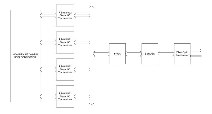
Mode 1 Block Diagram – Used in Back-to-Back mode to for a serial to fiber optic and back to serial extension product.
