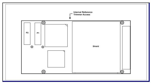
Figure 2.6.2. Reference Adjustment Access
