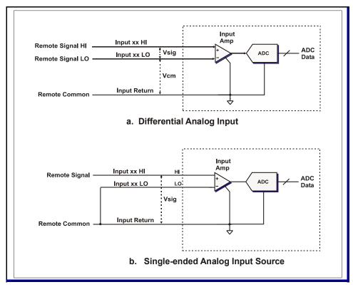
Figure 2.3.1. Input Configurations
