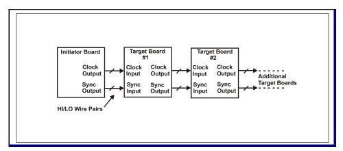
Figure 2.4.1. Multiboard Clock/Sync Connections
