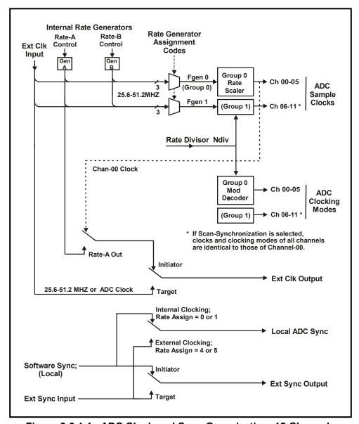
Figure 3.6.1.1. ADC Clock and Sync Organization, 12 Channels
