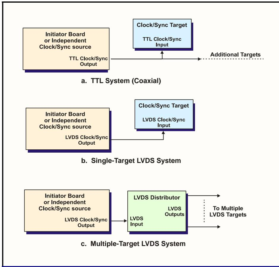
Figure 2.3-2. Multiboard Synchronization
