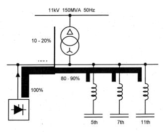
Harmonic filters consist of capacitors connected in series with a reactor. The capacitors produce reactive power at the filter's fundamental frequency, and the circuit is designed to achieve the required power factor correction. The inductance of the reactor is chosen so that the filter forms a very low impedance series resonant circuit at the harmonic frequency. This ensures that a high proportion of the harmonics enter the filter.
