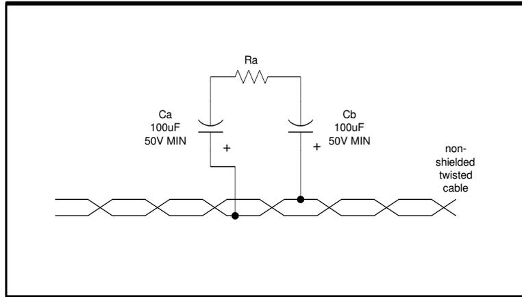
Figure 4-5: Typical termination of a network with twisted wire
