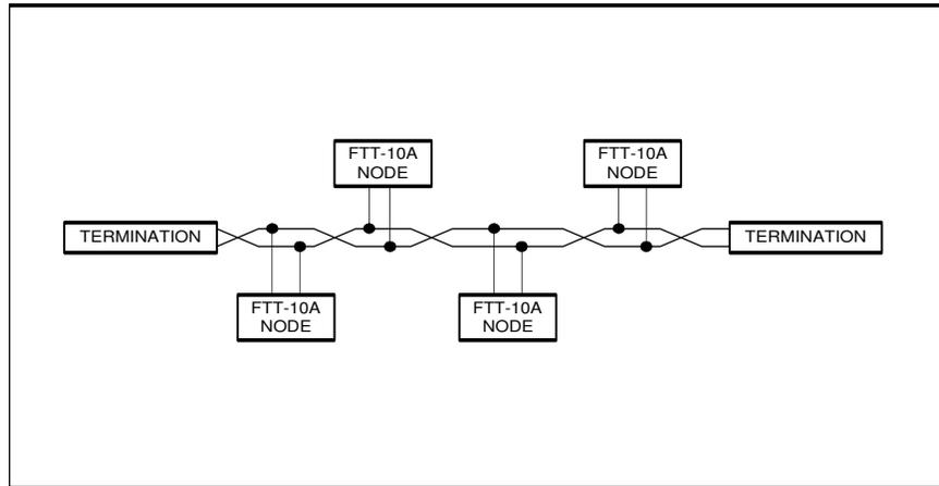
*Figure 4-3: Dual termination bus topology*
