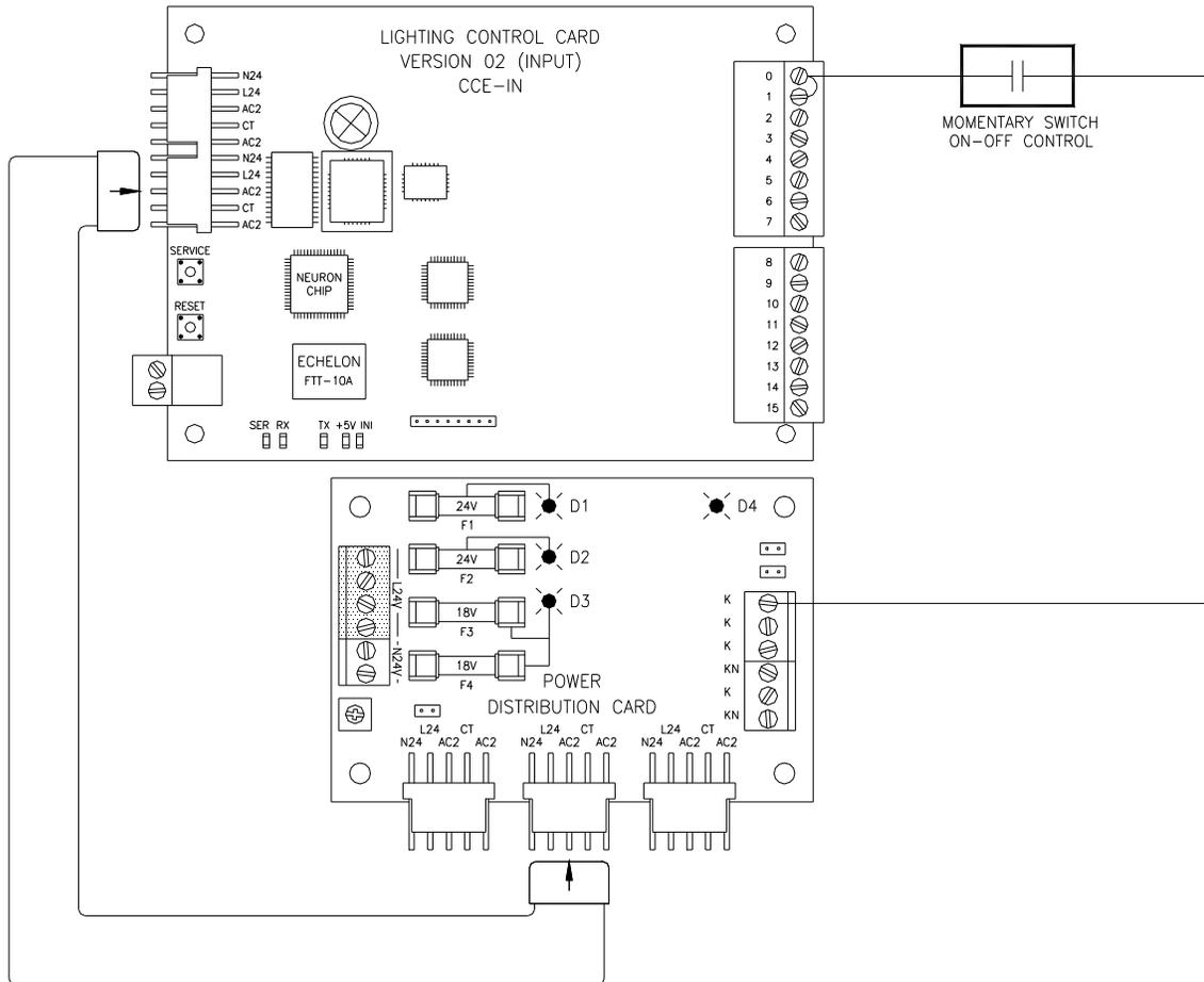
Figure 3-6: Momentary switch with ON-OFF control
