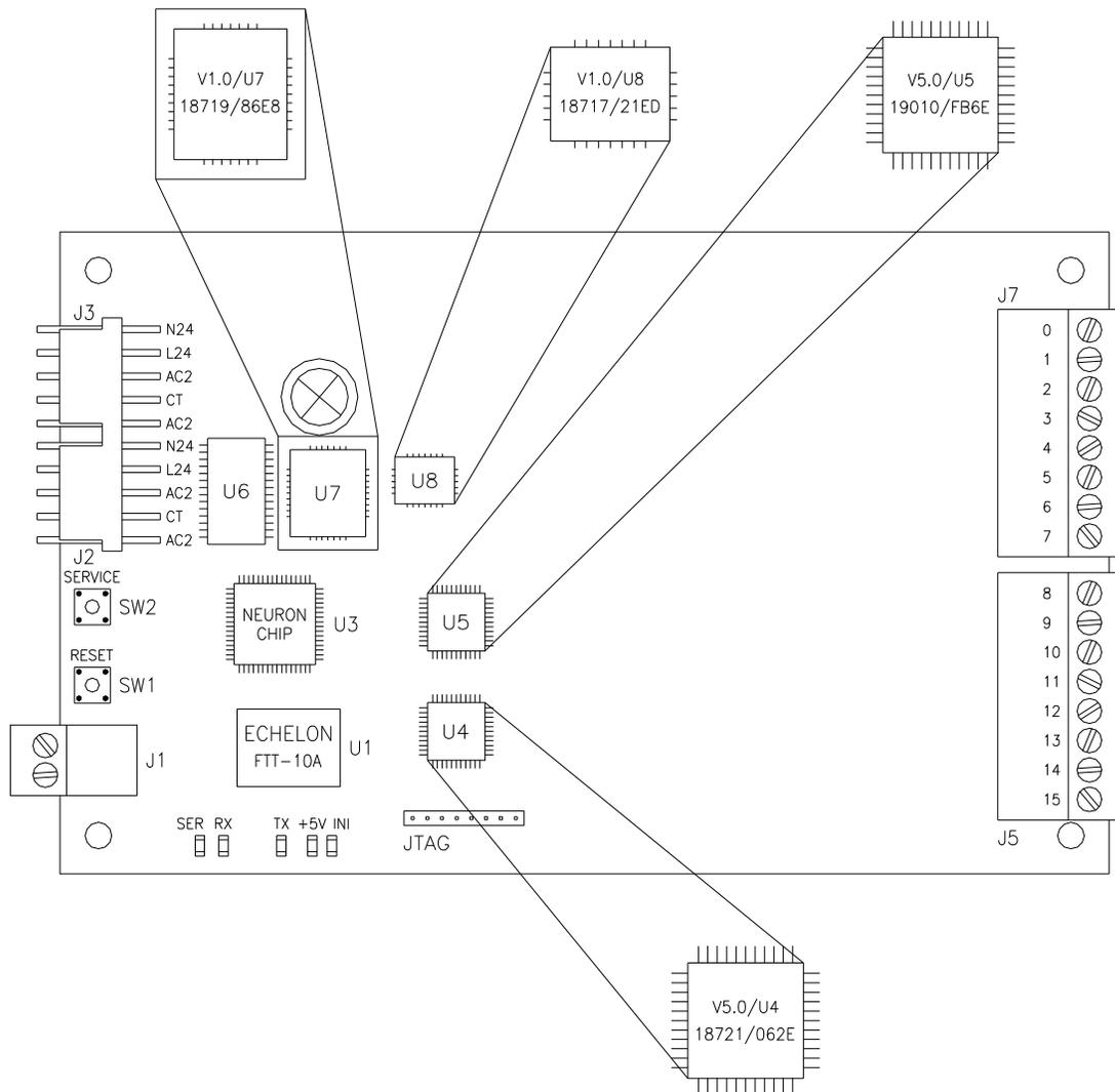
Figure 2-2: Lighting Control Card-Input (CCEIn)
