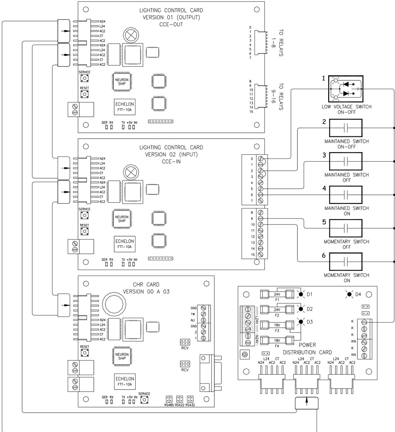
Figure 3-8: Interconnection diagram
