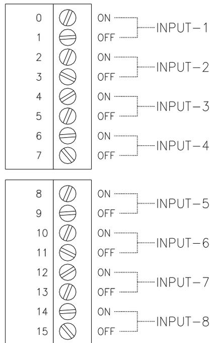
Figure 3-1: Connection of switches on an eight-input card
