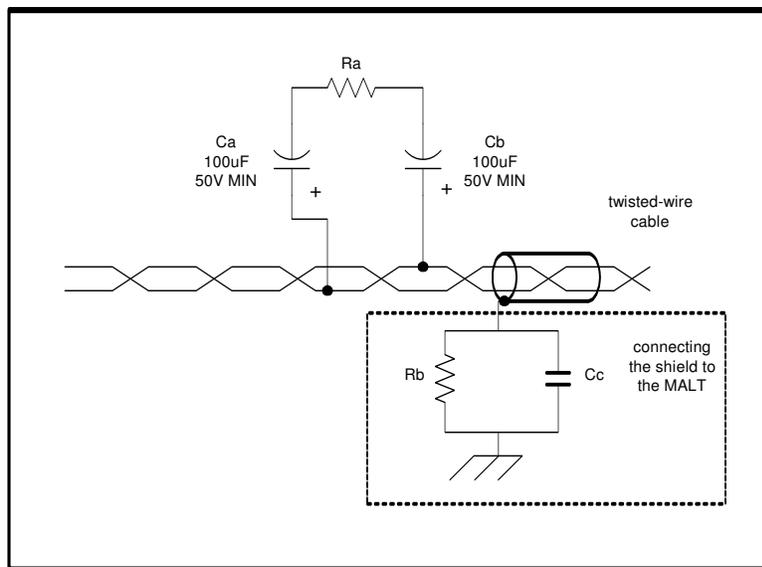
Figure 4-6: Connecting the shield to the ground
