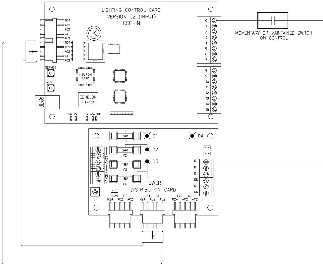
*Figure 3-4: Momentary or maintained switch with ON control*
