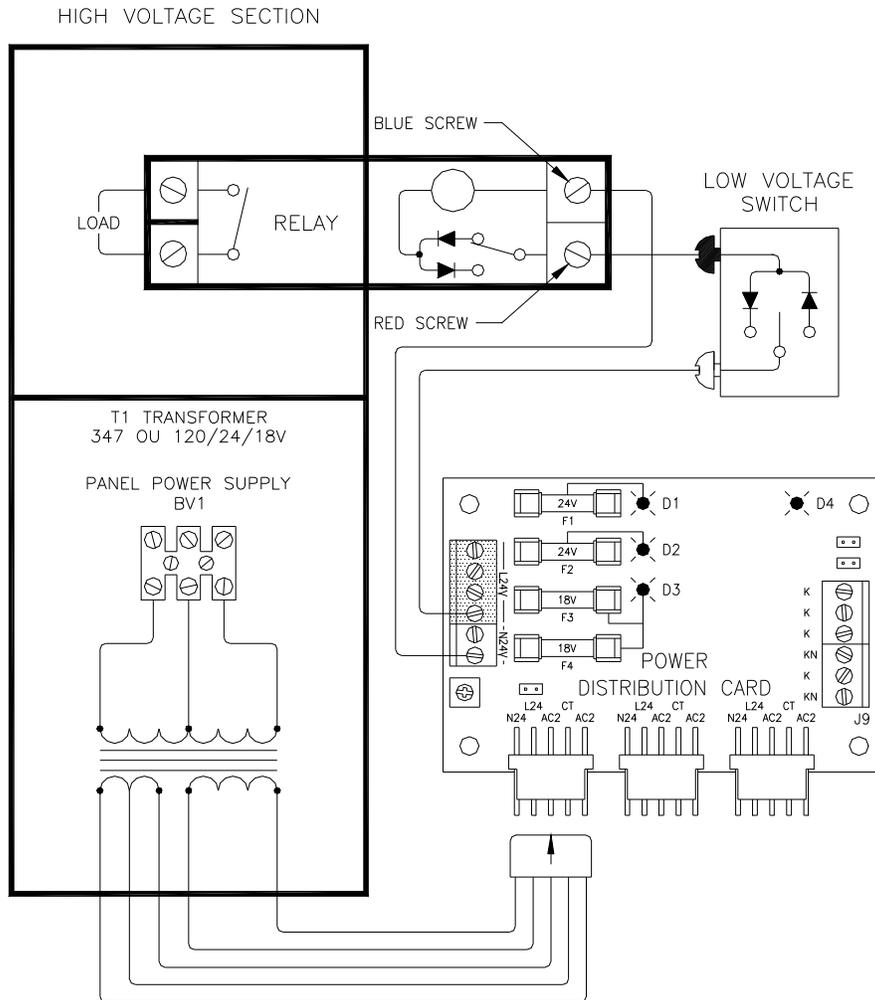
*Figure 3-7: Wiring diagram for two-wire relay*
