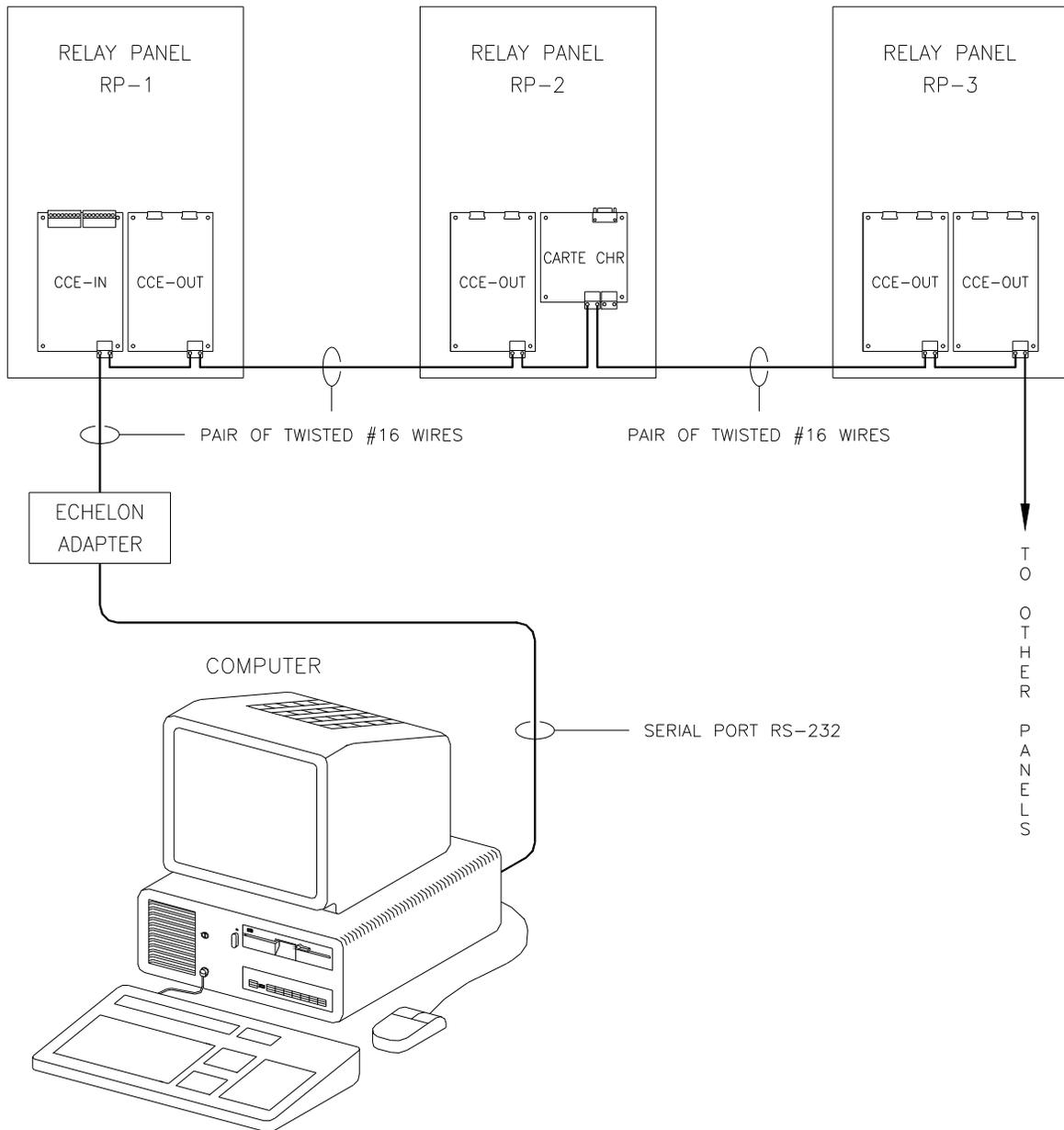
Figure 2-1: Typical Network Connection
