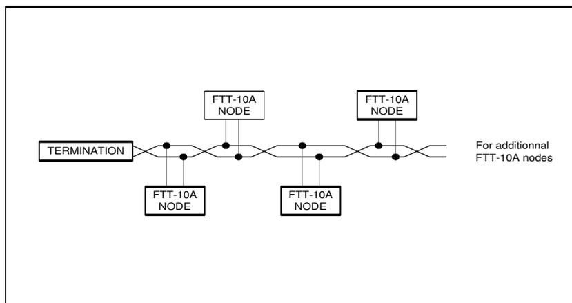
*Figure 4-2: Single termination bus topology*
