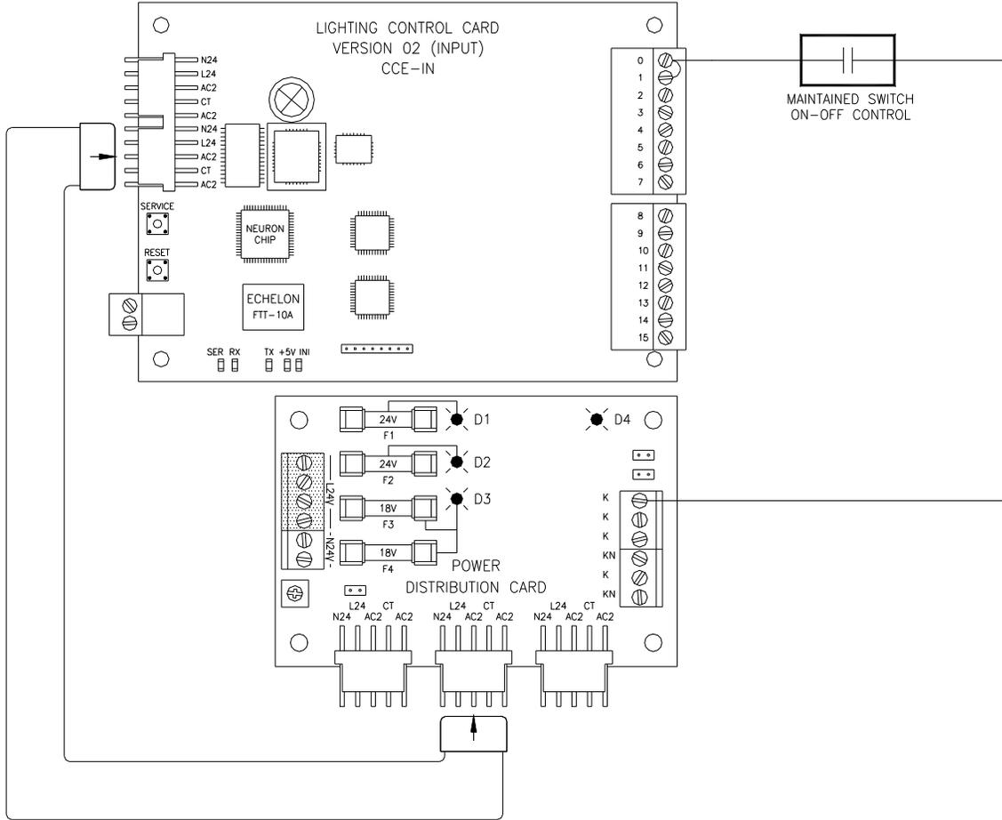
*Figure 3-3: Maintained switch with ON-OFF control*
