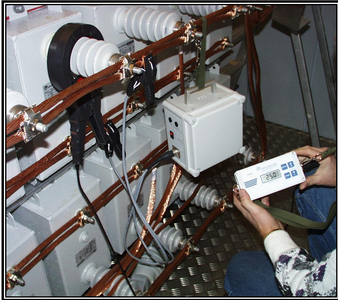
Fig. 7: Practical capacitor measurement
