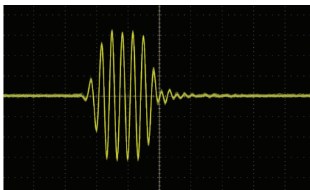
10 ns pulse at 750 MHz RF
