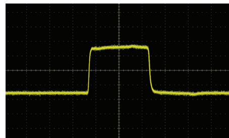
20 ns pulse envelope at 10 GHz RF
