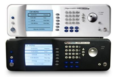
The Giga-tronics Model 2400 and 2500 Series Microwave Signal Generators are designed with several types of memory. The user-accessible memory is used to store various parameters pertaining to the synthesizer configuration, which include frequency, level parameters set by the user. There are 10 user-accessible memory locations for storing instrument states and 1 additional location reserved for recovering the last instrument state automatically stored when the synthesizer is powered down.
