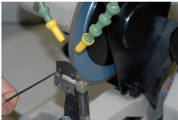
Knife rest and grinding wheel for sharpening blade in a Helicarb cutter on a Weing Rondamat Grinder or equivalent.
