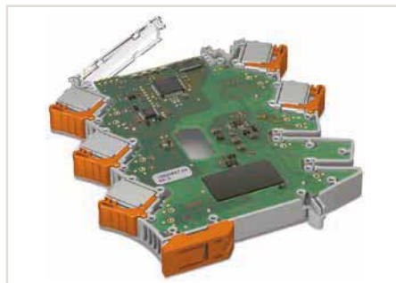
2. Insert and solder the PCB.
