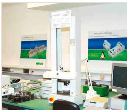
Conductor retention force testing
