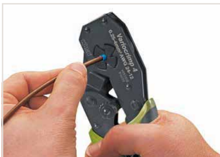
Squeeze handles until ratchet mechanism is released.
