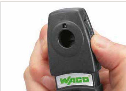
Set the cable diameter.
