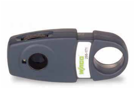
Cable stripper, for round cables with 2.5 mm ... 11 mm outer diameter
