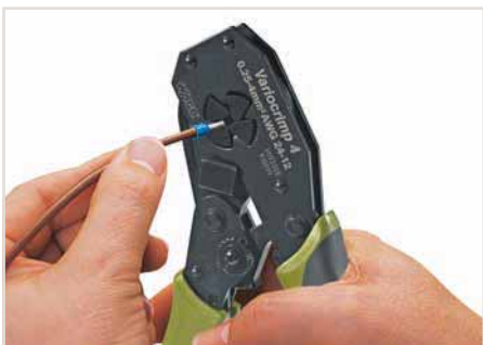
Insert ferruled conductor into the crimping station.
