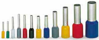
Ferrule, insulated, electro-tin-plated, electrolytic copper, gastight crimped, per DIN 46228, Part 4/09.90
