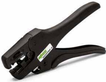
"Quickstrip 10" wire stripper, 0.02 ... 10 mm 2 "f-st" (6 mm 2 "s"), wire cutter f up to 10 mm 2 "f-st" (1.5 mm 2 "s")
