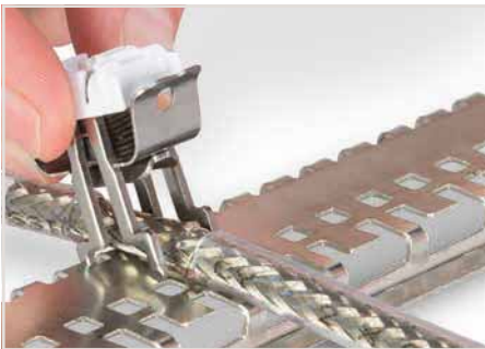
Mounting a clamping saddle on a specially slotted carrier rail (790-145). When releasing the saddle, do not place your finger under the clamping spring!
