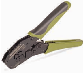
Variocrimp 4 crimping tool, for insulated and uninsulated ferrules, 0.25 mm 2 ... 4 mm 2 /AWG 24 ... 12
