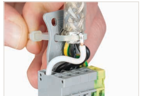
Fasten the shield conductor and the shield termination to the strain relief plate using cable ties.
