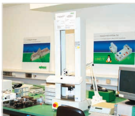
Conductor retention force testing
