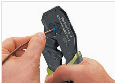
Squeeze handles until ratchet mechanism is released.
