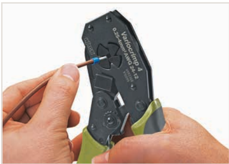
Insert ferruled conductor into crimping station.
