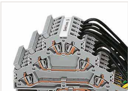
Commoning using comb-style jumper bars. Push comb-style jumper bars down until fully inserted. Group marking via marking strips (Item No. 709-177)
