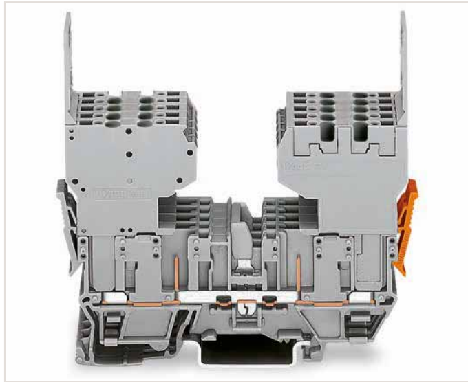
2 x 2-conductor female plugs Carrier terminal blocks can be commoned via 280 and 780 Series Jumpers and tested using a 280 Series Test Plug Adapter.
