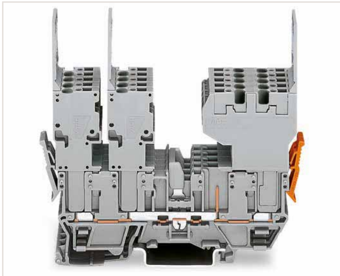
2 x 1-conductor female plug (left), 1 x 2-conductor female plug (right), may be reversed – carrier terminal blocks can be commoned via 280 and 780 Series Jumpers and tested using a 280 Series Test Plug Adapter.
