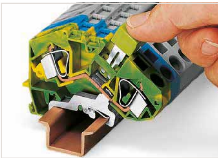
Commoning ground conductor terminal blocks with through terminal blocks is possible in one direction only (via rear side of terminal block) using adjacent jumpers. In addition to the required marking of these blocks, use yellow-green adjacent jumpers.
