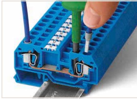
CAGE CLAMP® connection Inserting a conductor. With ferruled conductors, it is necessary to use a terminal block one size larger than the conductor's nominal cross-section.
