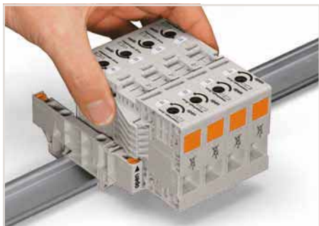
Removing the assembly: Turn the orange locking tab to the open position. Lift the assembly between the mounting adapters and remove it.
