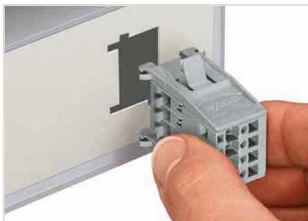
Insert male connector with snap-in flanges (769-604/005-000) into the cutout.
