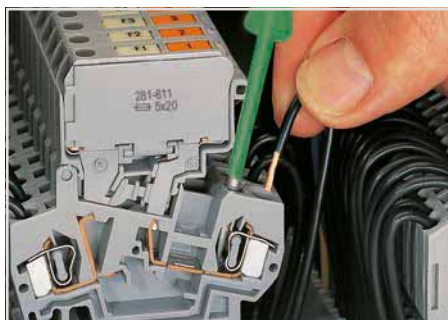
CAGE CLAMP® connection Inserting a conductor via screwdriver. With ferruled conductors, it is necessary to use a terminal block one size smaller than the conductor's nominal cross section.
