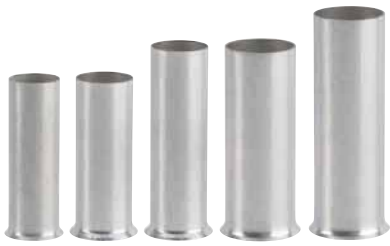
Ferrule, uninsulated, electro-tin-plated, electrolytic copper, gastight crimped, per DIN 46288, Part 4/09.90
