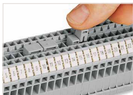
Commoning using an adjacent jumper (280-402). Push jumper down until fully inserted.
