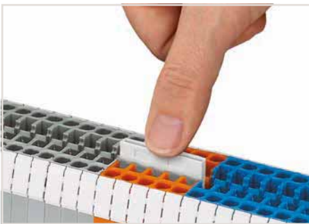
7 Push jumper bars down firmly until fully inserted. When using multipole bars, push alternately on the right and then left side, until installed. Push-in type jumper bars 1-3-5-7 or 1--4--7 upon request
