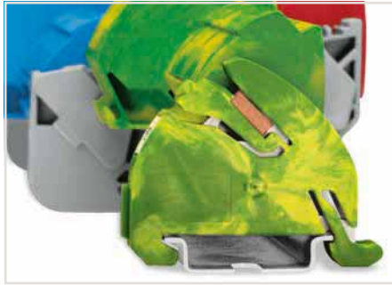
Ground busbar carrier (812-141): Offers a receptacle with locking device for (10 x 3) mm busbar. Contact between the busbar and rail is made automatically by simply snapping the carrier onto the DIN-35 rail. One end of the busbar is mounted onto the ground busbar carrier, the other end is inserted into the middle position of the insulated busbar carrier.
