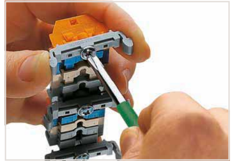
Terminal strip with mounting flanges – screwing a 209-123 Mounting Foot (distance between mounting feet: approx. 25 ... 30 mm)
