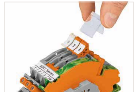
Using locking covers or profiles for adjacent terminal blocks allows disconnect links to be operated simultaneously.
