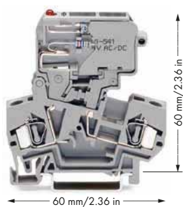
Fused disconnect terminal block with a pivoting fuse holder, with blown fuse indication by LED, gray, for (5 x 20) mm miniature metric fuse
