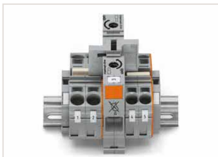
Commoning 35 mm 2 (2 AWG) POWER CAGE CLAMP Terminal Blocks with 10/16 mm 2 (8/6 AWG) TOPJOB® S Terminal Blocks using step-down jumpers (285-430).
