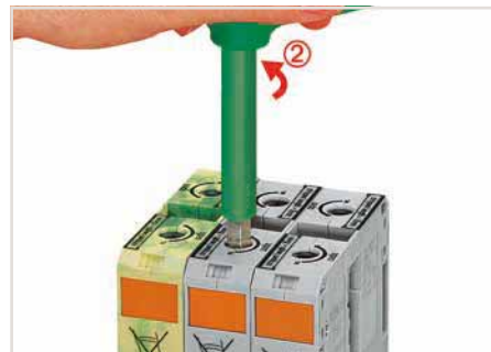
Conductor termination – step 3 A short counter-clockwise rotation ② releases the locking tab. When unlocked, the T-wrench rotates clockwise, securely clamping the conductor.
