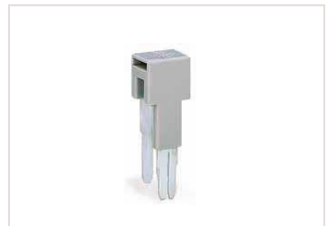
Step-down jumper from 16 mm 2 (6 AWG) to 4 mm 2 (12 AWG); I N 32 A, Item No. 283-414
