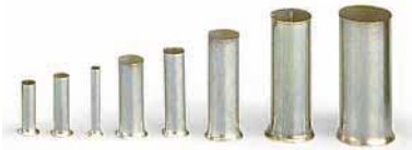
Ferrule, uninsulated, electro-tin-plated, electrolytic copper, gastight crimped, per DIN 46288, Part 4/09.90
