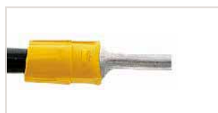
Crimped pin terminal (gas-tight), preferably made of copper with a tin-plated surface
