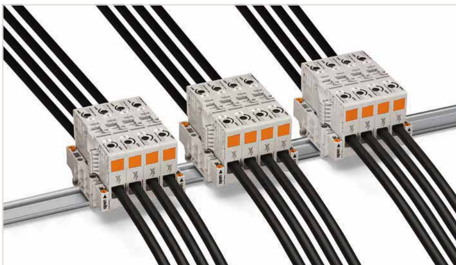
Removing the assembly: Turn the orange locking tab to the open position. Lift the assembly between the mounting adapters and remove it.
