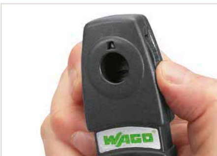
Set the cable diameter.
