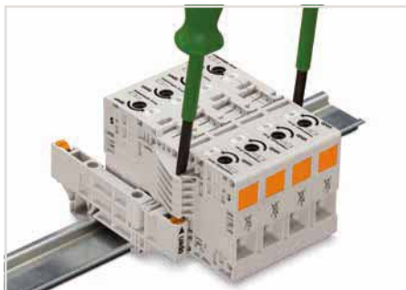
Removing the assembly: Insert two operating tools into the separator slots between male and female connectors and unlatch the assembly.
