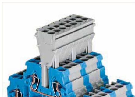
Three anti-reverse mating modules are necessary when snapping more than seven modules together.
