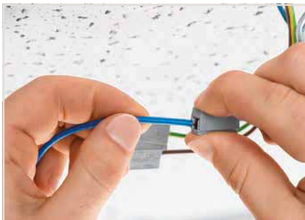
To connect: Press button fully, insert stripped conductor into square entry and release.
