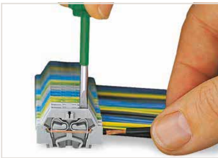
CAGE CLAMP® connection Inserting a conductor via screwdriver. With ferruled conductors, it is necessary to use a terminal block one size larger than the conductor's nominal cross-section.
