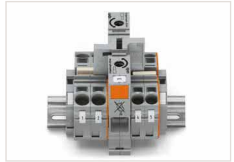
Commoning 35 mm 2 (2 AWG) POWER CAGE CLAMP Terminal Blocks with 10/16 mm 2 (8/6 AWG) 2010 and 2016 Series TOPJOP® S Terminal Blocks using step-down jumpers (not valid for 2016-76xx and 2016-77xx).
