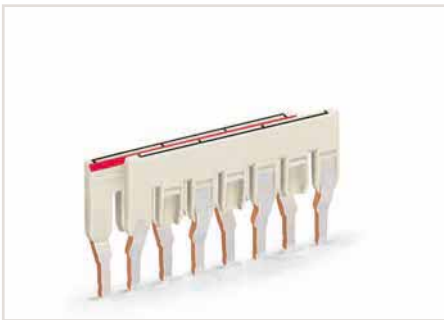
Locate red stripes of the staggered jumpers on the inside. Insert staggered jumper and push down until it hits backstop. Custom staggered jumpers can be created, e.g., for bridging over a terminal block with a different potential.
