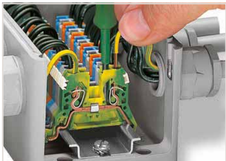
CAGE CLAMP® connection Inserting a conductor via operating tool (0.08 ... 4 mm 2 "f-st"). With ferruled conductors, it is necessary to use a terminal block one size smaller than the conductor's nominal cross section.
