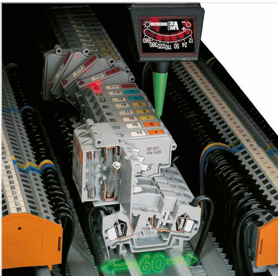
CAGE CLAMP® connection Inserting a conductor via screwdriver. With ferruled conductors, it is necessary to use a terminal block one size smaller than the conductor's nominal cross section.
