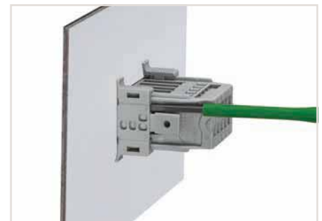
For removal, insert operating tool (2.5 mm blade) into release slot.
