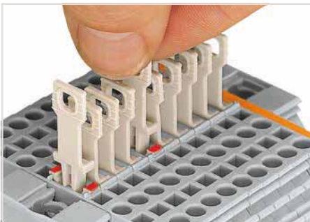
Pulling the disconnect tab by hand.
