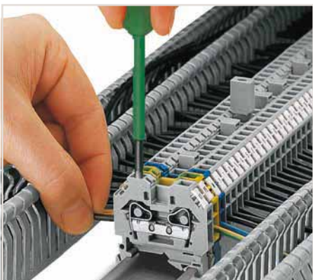
CAGE CLAMP® connection Inserting a conductor via screwdriver. With ferruled conductors, it is necessary to use a terminal block one size larger than the conductor's nominal cross-section.
