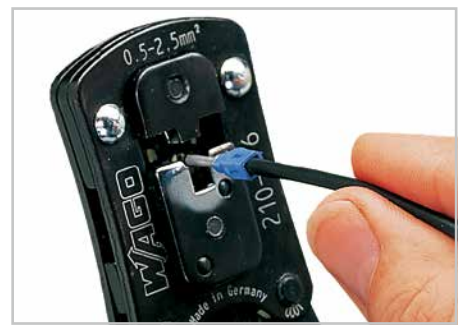
Squeeze the crimping tool beyond the lock-in position, then remove the conductor with crimped pin terminal.
