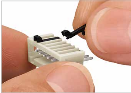
Coding a male header - fitting coding key(s).
