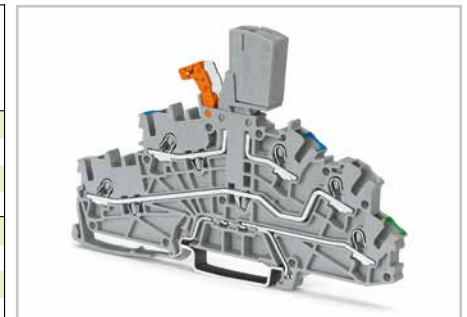
2003-6641 Multilevel Installation Terminal Block with 2003-499 N/L Test Plug Adapter for insulation resistance measurement with connected N and L potentials
