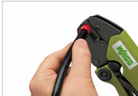
Squeeze handles until ratchet mechanism is released.
