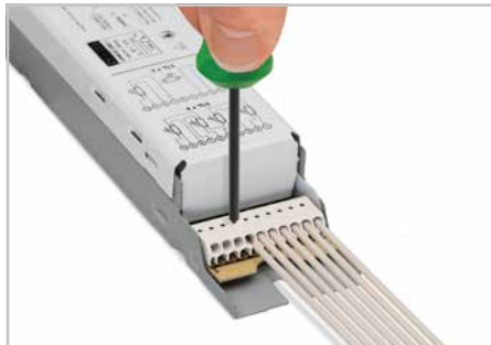
Removing a conductor by inserting disconnection tool into the operating slot and pulling it out.
