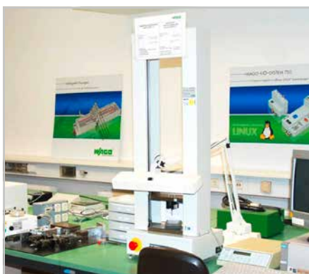
Conductor retention force testing
