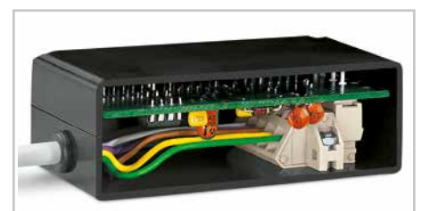
Panel-mount connectors Pictures shows a male connector with CAGE CLAMP® and strain relief plate for outgoing circuit.
