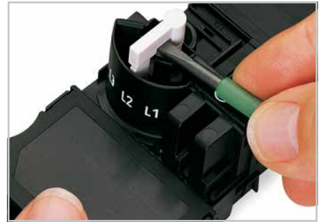
Lift jumper out of delivery position (L2) using a screwdriver and move it into the desired position.
