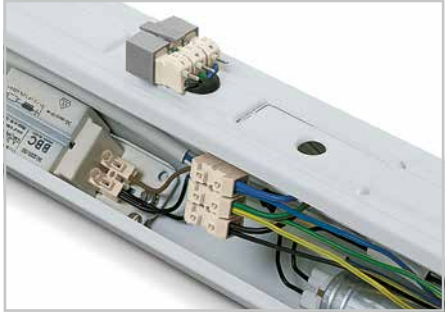
Lighting fixture ready for connection with center receptacles (internal wiring complete with WAGO terminal blocks)
