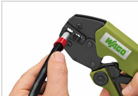
Insert ferruled conductor into crimping station.
