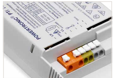
WAGO's 804 Series Terminal Strips provide "internal commoning" to meet requirements that ban routing the ground conductor over the board. This enables custom terminal strips to be commoned and marked at the factory upon request.
