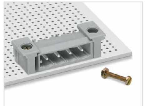
M 2 x 12 screws with nut (e.g., for locking devices)
