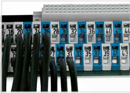
PCB Terminal Strips placed behind each other save space – staggering them by half the pin spacing simplifies subsequent wiring of the first row.
