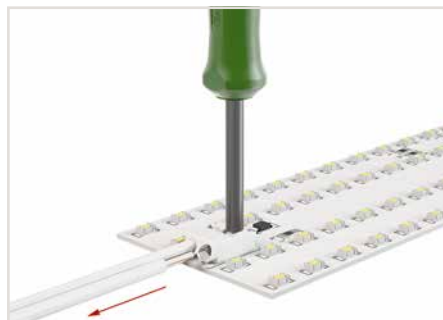
Inserting/removing fine-stranded conductors by lightly pressing on a push-button (e.g., via 206-861 Operating Tool).
