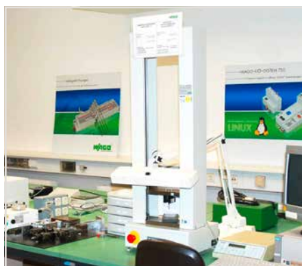
Conductor retention force testing
