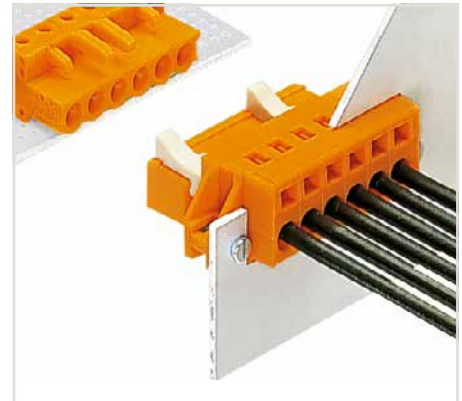
Self-tapping screws, for 1.8 mm ± 0.1 mm Ø mounting hole
