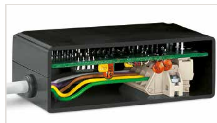
Angled female plug – a male header with straight solder pins is used for horizontal PCB mounting in narrow housings.
