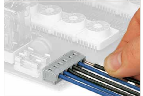
Inserting a solid conductor via push-in termination.
