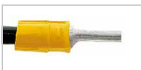
Crimped pin terminal (gas-tight), preferably made of copper with a tin-plated surface
