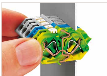
Insert the terminal strip into the cutout until the stop hits the enclosure wall.
