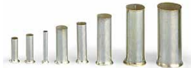
Ferrule, uninsulated, electro-tin-plated, electrolytic copper, gastight crimped, per DIN 46288, Part 4/09.09
