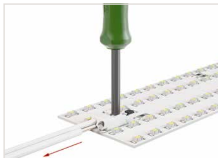
Insert/remove fine-stranded conductors by lightly pressing on push-button (e.g., via 206-861 Operating Tool).
