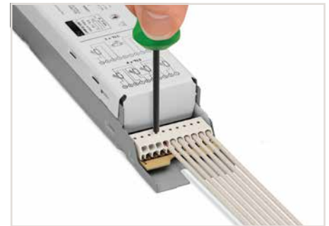
Removing a conductor via 1.0 mm \varnothing disconnection tool (206-840).
