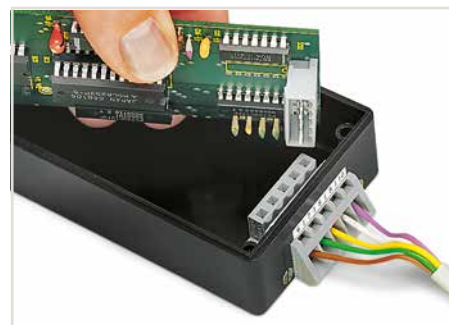
Angled female connector used as through-panel connector. Termination ports and operating slots are located outside the housing – panel thickness up to 2 mm.
