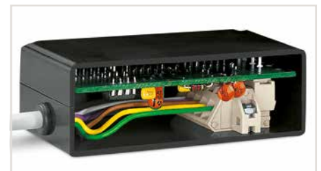
Angled female plug – a male header with straight solder pins is used for horizontal PCB mounting in narrow housings.
