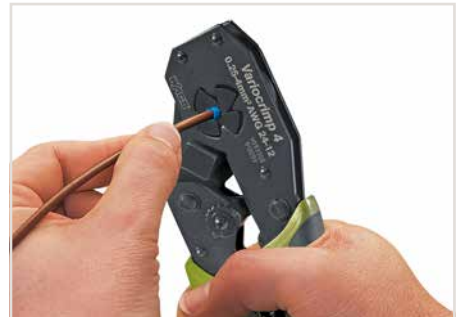
Squeeze handles until the ratchet mechanism is released.
