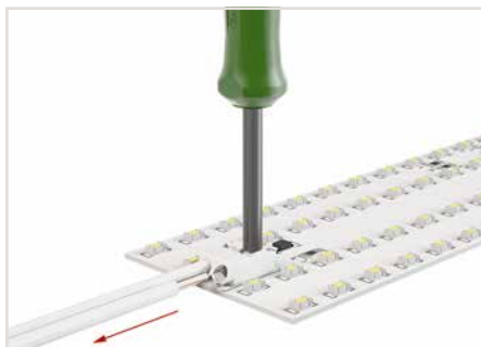
Inserting/removing fine-stranded conductors by lightly pressing on a push-button (e.g., via 206-860 Operating Tool).
