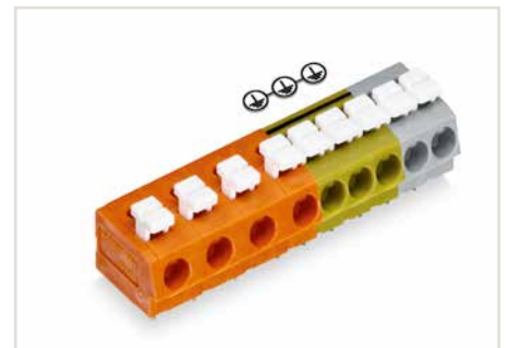
WAGO's 804 Series Terminal Strips provide "internal commoning" to meet requirements that ban routing the ground conductor over the board. This enables custom terminal strips to be commoned and marked at the factory upon request.
