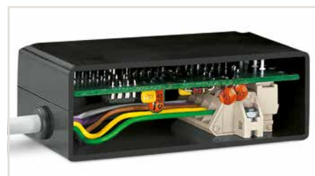
Angled female plug – a male header with straight solder pins is used for horizontal PCB mounting in narrow housings.
