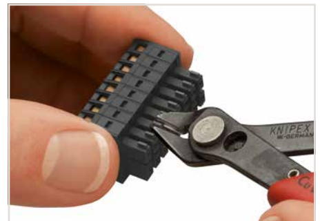
Coding a female connector – removing coding finger(s).
