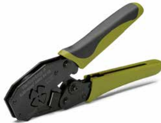
"Variocrimp 4" crimping tool, for insulated and uninsulated ferrules, crimps 0.25 ... 4 mm 2 conductors
