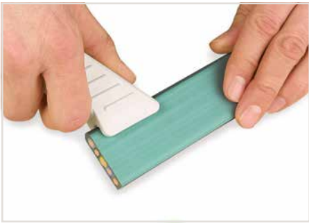
Cut both sides of the flat cable insulation using a stripping knife (observe 30 mm of cutting length).
