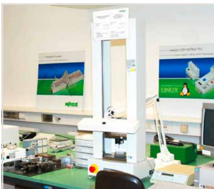
Conductor retention force testing
