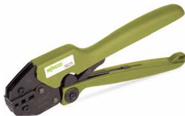
Crimping Tool 25, for insulated and uninsulated ferrules, crimping range: 10 mm 2 , 16 mm 2 and 25 mm 2
