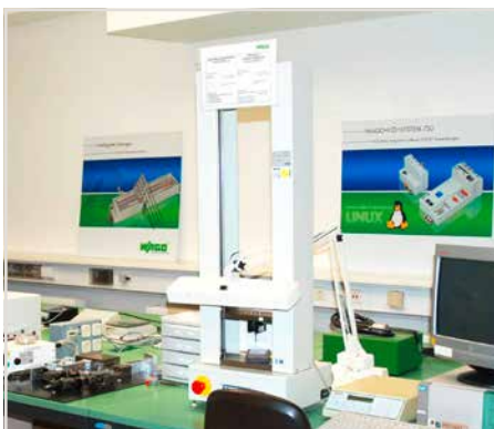
Conductor Retention Force Testing
