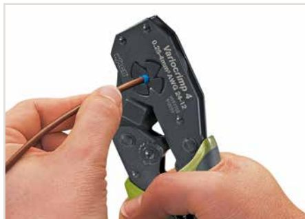
Squeeze handles until ratchet mechanism is released.
