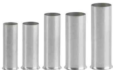
Ferrule, uninsulated, electro-tin-plated, electrolytic copper, gastight crimped, per DIN 46288, Part 4/09.90
