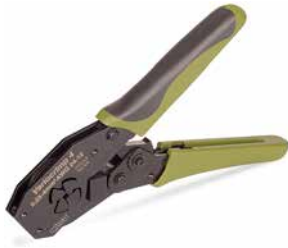
„Variocrimp 4“ crimping tool, for insulated and uninsulated ferrules, 0.25 ... 4 mm 2 /24 ... 12 AWG
