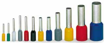
Ferrule, insulated, electro-tin-plated, electrolytic copper, gastight crimped, per DIN 46288, Part 4/09.09
