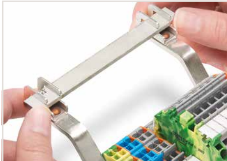
Place the busbar in the busbar carrier.
