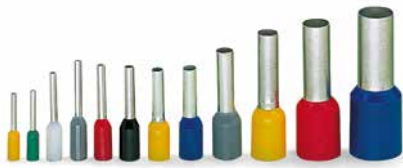
Ferrule, insulated, electro-tin-plated, electrolytic copper, gastight crimped, per DIN 46288, Part 4/09.09
