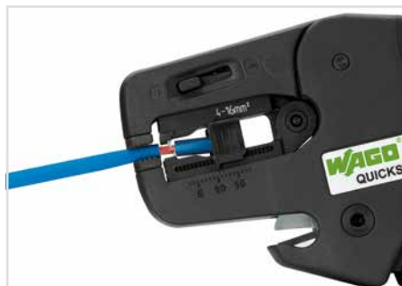
Stripping a conductor.
