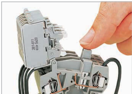
Distributing current to several fuse-protected circuits via insulated touch-proof jumpers.
