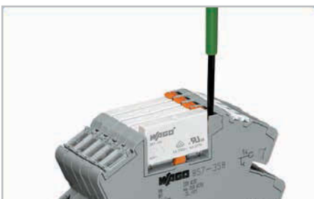
Removing a relay via ejector.
