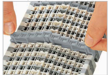
Grip end plate at both sides and – push down (assembly) – pull up (removal)
