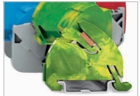
Carrier including a receptacle with locking device for (10 x 3) mm busbar. Contact between the busbar and rail is made automatically by simply snapping the carrier onto the carrier rail. One end of the busbar is mounted onto the ground busbar carrier, the other end is inserted into the middle position of the insulated busbar carrier.
