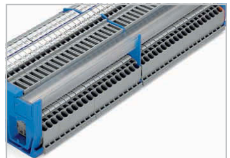
The compact busbar carrier, which is placed every 200 mm, provides additional busbar support for longer assemblies.
