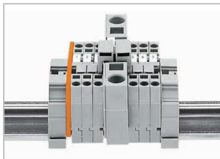
Commoning from 16 mm 2 (283 Series) to 4 mm 2 (281 Series) rail-mounted terminal blocks via step-down jumpers.
