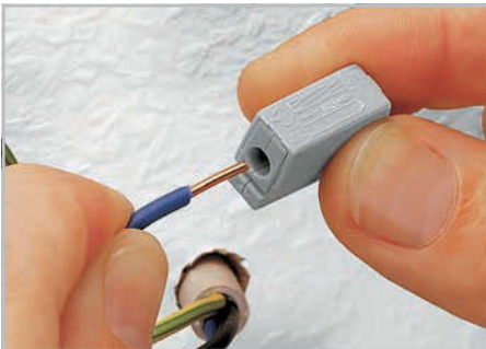
Installation side: Insert stripped solid conductor into circular entry and push until it hits the backstop.
