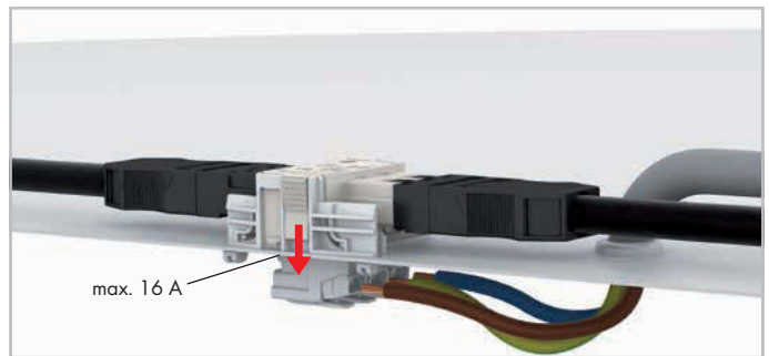
WAGO Linect® Lighting Terminal Blocks are ideal for connecting additional consumers that were not originally planned (e.g., spots). The maximum current between WINSTA® Linect® T-Connector and Lighting Terminal Block is 16 A.
