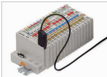
Accessing the programming interface - Programming a fieldbus controller WAGO-I/O-CHECK, WAGO-I/O-PRO CAA.
