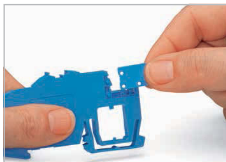
Inserting the separator plate to protect the N-busbar against accidental contact.
