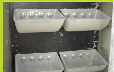
Starco Jumbo Buckets on 4B Steel Web Core Belt Cement Application
