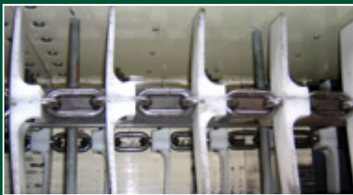
Bolt 'N' Go System Round Link Chain Application on a Conveyor
