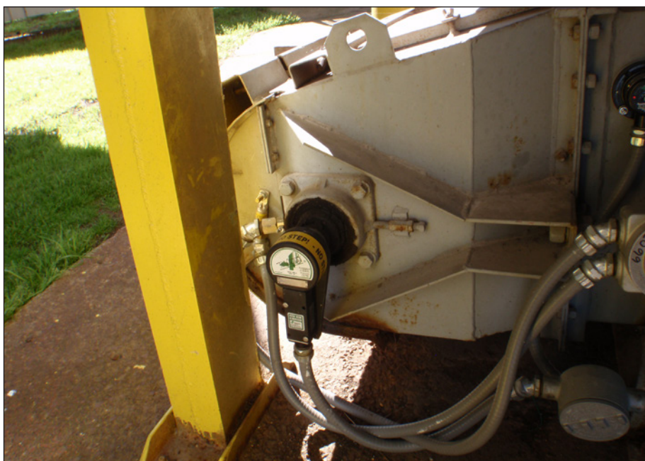
Whirligig® Installed on the Tail Shaft of Enclosed Conveyor with M800 Elite Speed Switch
