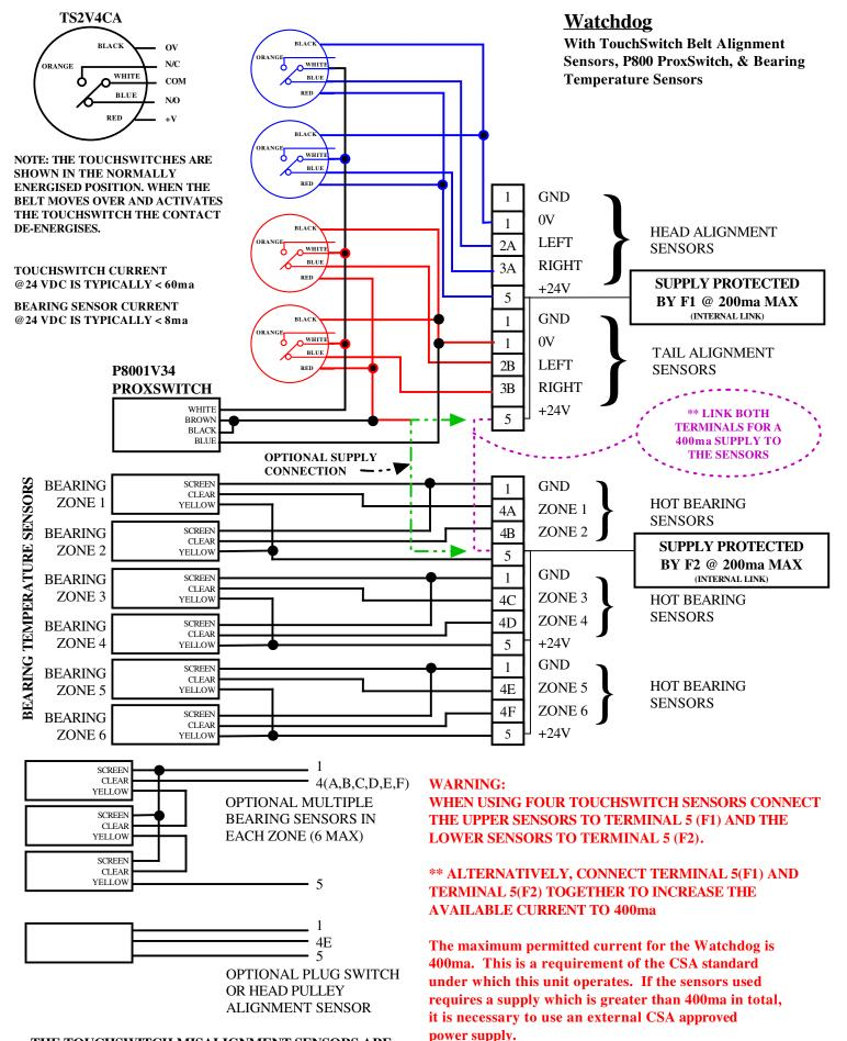
THE TOUCHSWITCH MISALIGNMENT SENSORS ARE DESIGNED TO IMMEDIATELY STOP THE BELT WHEN THEY ARE TOUCHED BY THE MISALIGNED BELT. THEREFORE THE MISALIGNMENT AND PERSISTENT ALARM DELAY SHOULD BE REDUCED TO ZERO.
