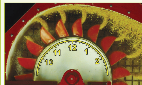
4B Test Elevator showing initial centrifugal discharge (10 o'clock) with Starco buckets handling dry corn.
