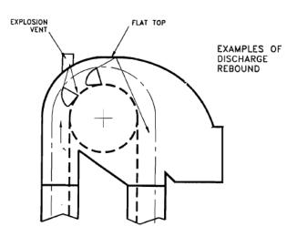
Centri-gravity discharge is normally used for discharging powders, pellets, cement and fragile materials at slow speeds. The buckets start to discharge at top dead center (12 o'clock) and continue until approximately 50° afterwards. Recommended bucket types for centri-gravity discharge are Super Starco Steel and Starco Jumbo (SJ) buckets.
