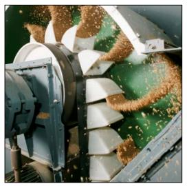
Centrifugal Discharge of CC-S Buckets Shown Handing Grain
