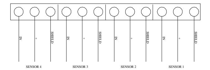
The TN4 has been designed to be HOT swappable (**Division 2 only**). The terminals are plug-in types to allow the user to remove a faulty board and replace it without disturbing the rest of the installation and whilst the equipment is still live. If you intend to make wiring changes or if the TN4e is installed in a **Division 1** environment, you MUST first disconnect power from the system to ensure that you eliminate the risk of electrical shorting on live conductors.
