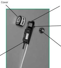
Cup Target (1, 2, 4, or 8 targets for shaft speed detection)
