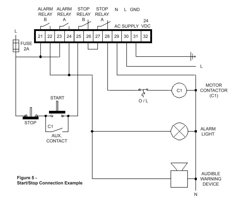
Figure 5 is an example showing a conventional start/stop circuit wired for driving the motor contactor. In this case, the stop relays are wired in series and the alarm relays are wired in parallel.
