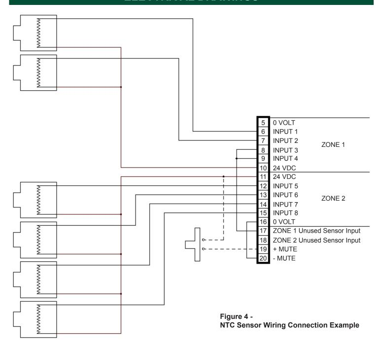
Figure 4 shows the connection of 2 NTC temperature sensors to zone 1 inputs 1 and 2.
