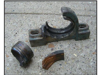
Example of Bearing Failure
