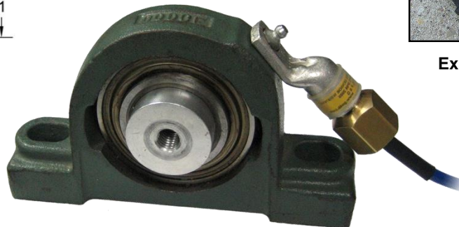
WDB70V3C Installed on Bearing Housing
