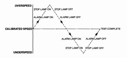
The TEST function can be performed at any time whether the machine is running or stationary; as the relays do not operate from the TEST function, the normal running of the machine is unaffected. If, during the TEST function, a real ALARM or STOP condition occurs, the relevant relay will operate
