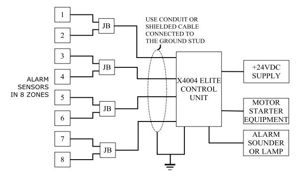
Drawing B: DC Supply Connections with AC/DC Motor Circuit
