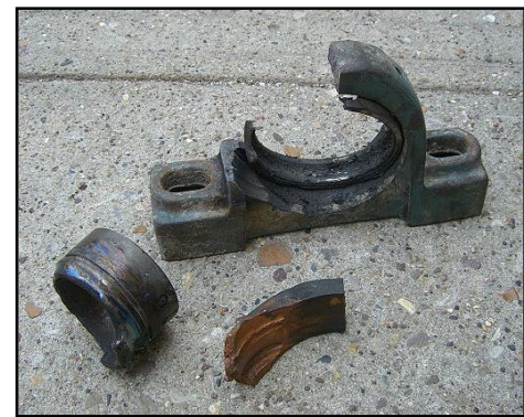
Example of Bearing Failure
