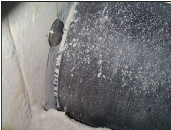
Touchswitch installed at the drive end of an enclosed belt conveyor (inside view).
