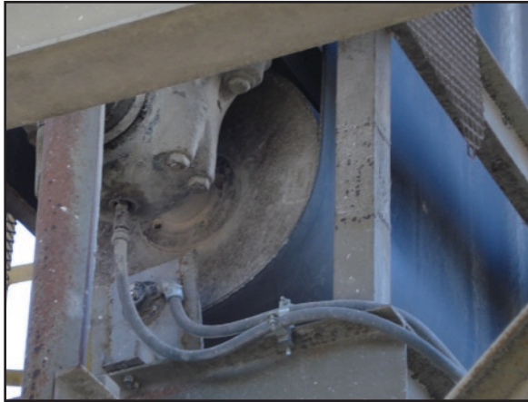
Touchswitch installed on take-up pulley of an open belt conveyor.
