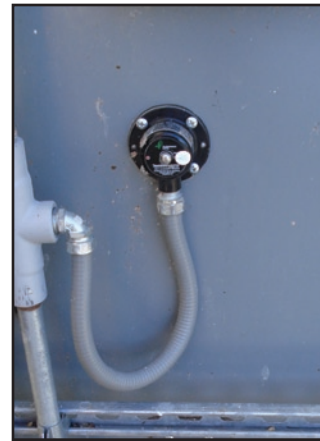
Touchswitch installed on a bucket elevator.
