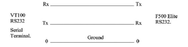
On more recent versions of the F500 TB1 may be a standard 9 pin Dee connector. This Dee connector is designed to work with a standard 9 pin to 9 pin serial lead for monitoring the F500
