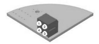
Led 1 Status Not used in this version of the Fieldbus module.
