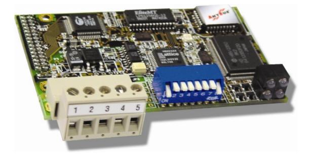
The above picture shows the location of the main parts of the DeviceNet Fieldbus module.
