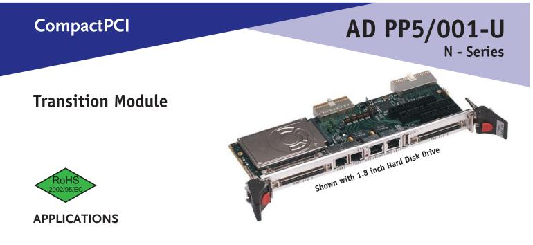
The AD PP5/001-U is designed to be used with Concurrent Technologies' PP 41x/03x, PP 33x/02x-U and PP 31x/01x-U CompactPCI® Processor board families. The Transition Module mounts in the rear transition area of the CompactPCI backplane and provides very simple access to the majority of the I/O functions provided on the processor board. Many I/O interfaces are accessed through the Transition Module's own front panel and the remainder from headers mounted on the Module.
