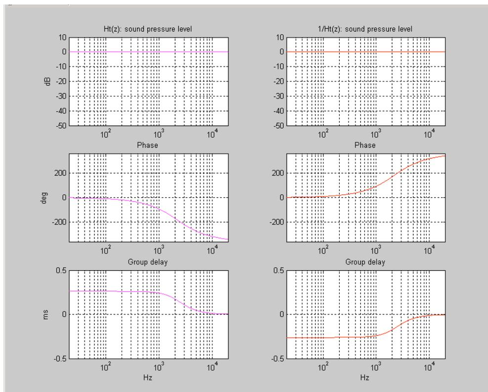
As we can see, the result of the summation of group delays is equal to zero. The group delay distortion has then been properly corrected.
