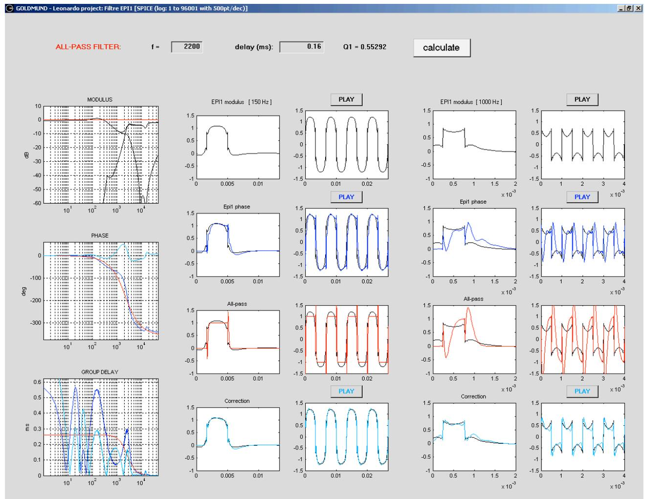
As explained above, the correction of the Epilogue 1 group delay distortion comes from the multiplication of its all-pass crossover by the inverse of the chosen all-pass filter (coefficient inversion).
