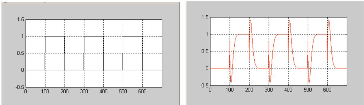
It is worth noting that the amplitude frequency responses of these two signals are absolutely identical. The sole difference comes from the phase response behaviour.
