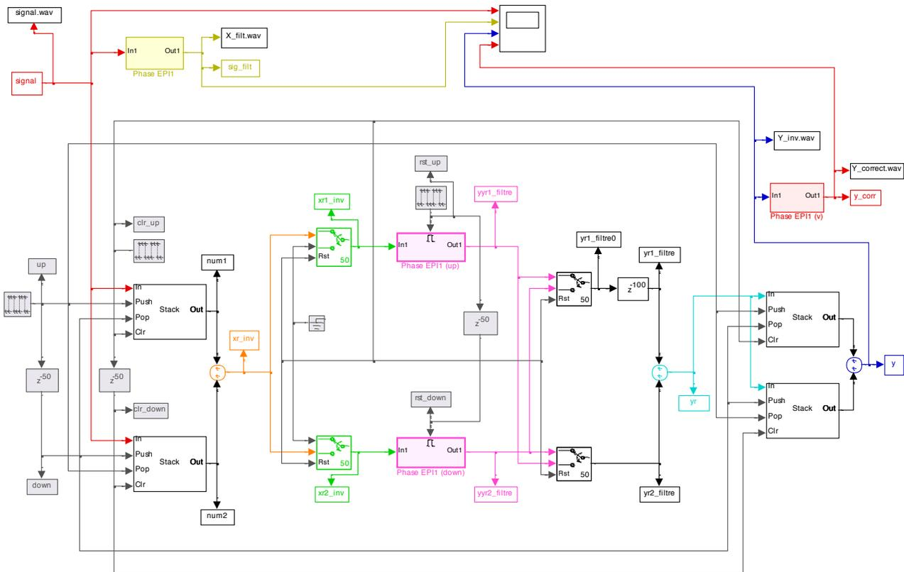
The input signal is acquired in consecutive sections of the length  $L$  samples. The sections are time reversed (input LIFO buffers) and separated in two signals (the sections are taken half the time and completed by zeros to form sections of the length  $2L$  samples).
