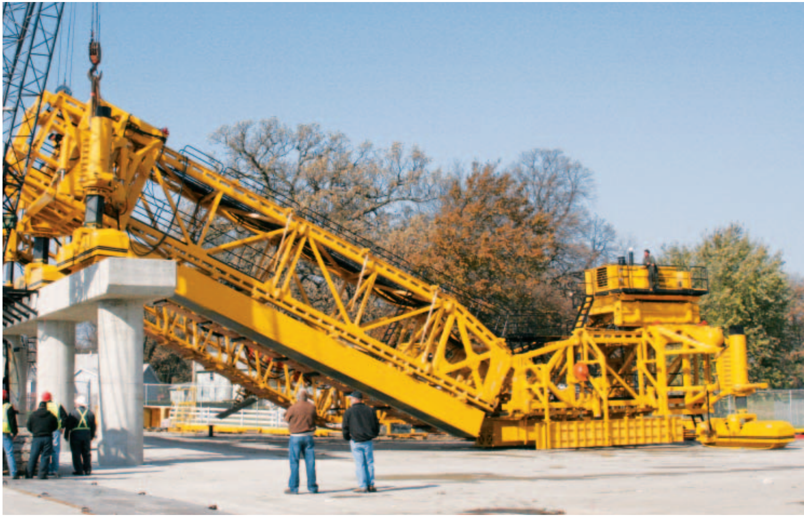
The All-American Canal paver features framework that is 10 feet (3 m) tall with a GP-4000 prime mover. It also has a powered wedge that allows the paver to be adjusted to the different angles caused by the changing widths and slopes of the canal.
