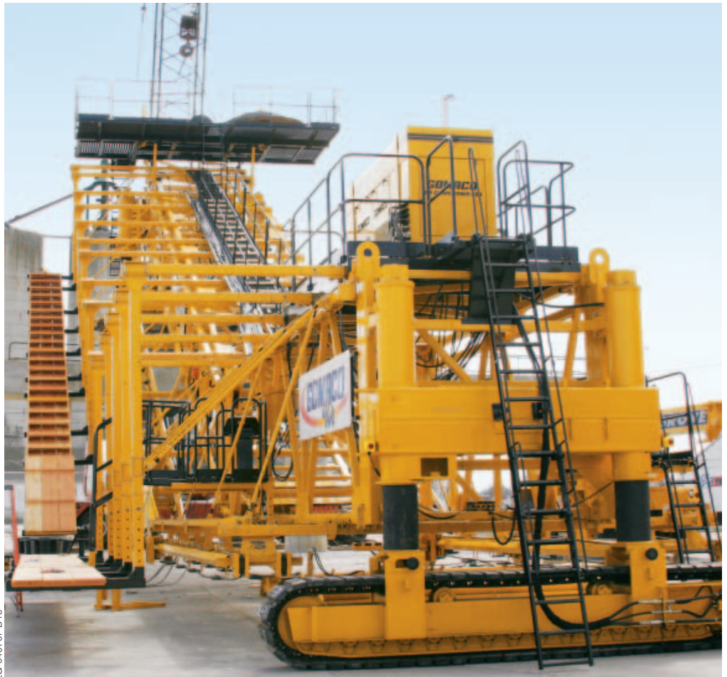
The water stop inserter machine has a specially designed inserter mechanism to place the rubber water stop material into the concrete every 15 feet (4.6 m) to form the transverse joint.
