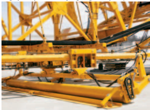
A 17 foot (5.2 m) long finishing cylinder with float pan will finish and seal the surface of the canal.
