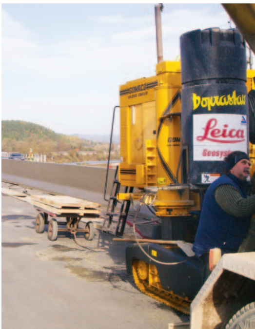
The GT-3600 is equipped with Leica's PaveSmart system for stringless paving.
