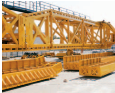
Modified 5000 series paving molds wait to be attached to the canal paver during assembly.
