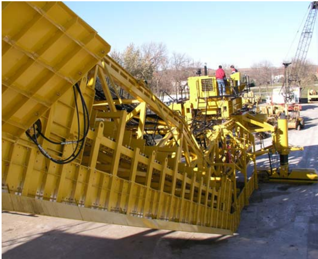
On the testing pier— the pier simulates the slope of the canal and allows engineers to test the different features on all three pieces of canal equipment.
