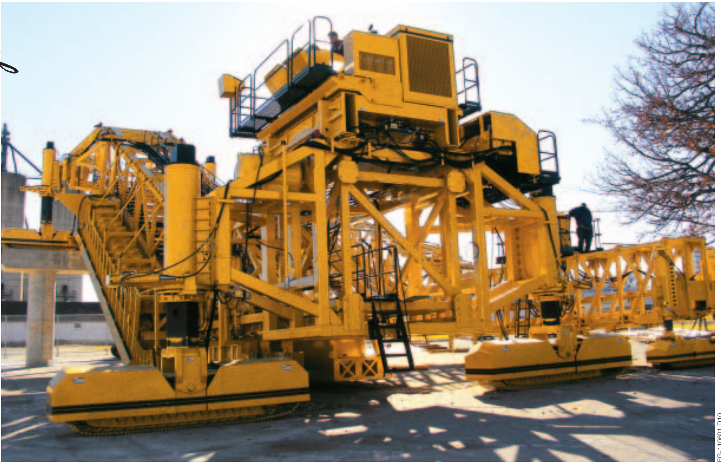
The paver and work bridge for the All-American Canal sits on the pier at GOMACO's testing facilities in Ida Grove, Iowa.
