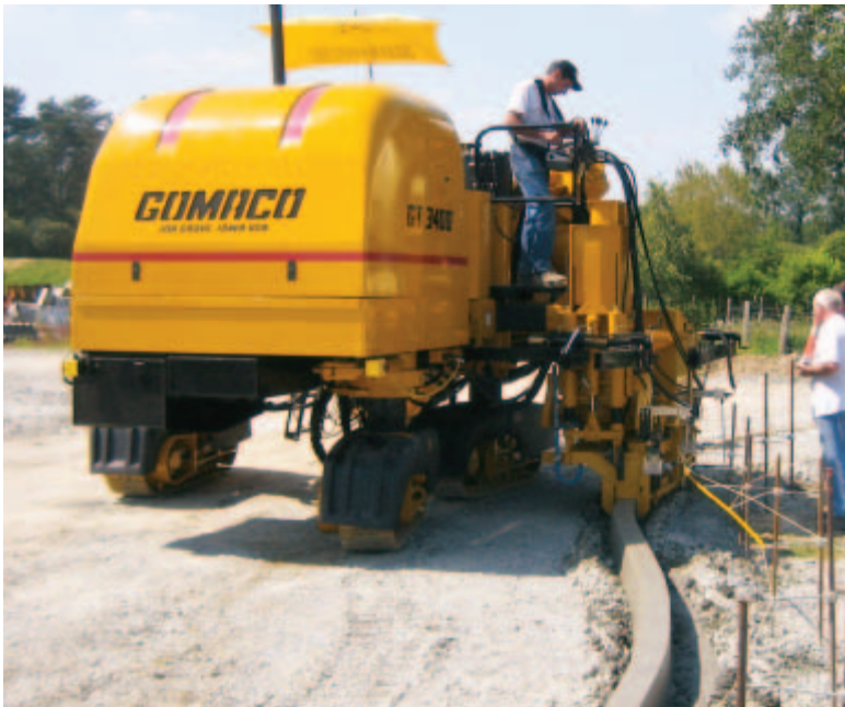
LBR takes advantage of their new GT-3400's right-side slipforming capabilities in Savenay, France. The machine's new G22 dual language capabilities allow the operator to operate the machine in his own French language.
