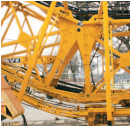
The powered wedge system allows the machines to go from flat to varying degrees of slope.
