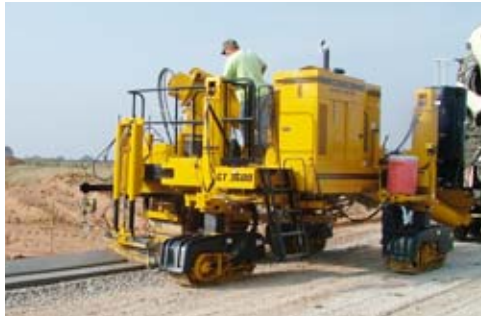
The company slipformed 11,000 feet (3353 m) of rollover curb on a new subdivision project.
