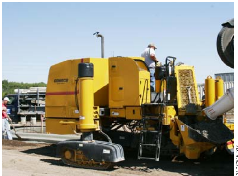
The GT-3400 turned several tight radii on a curb and gutter parking lot project in Faribault, Minnesota.
