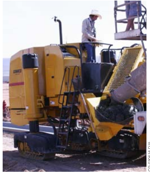
The new footprint has two close tracks on one side and a single track on the other.
