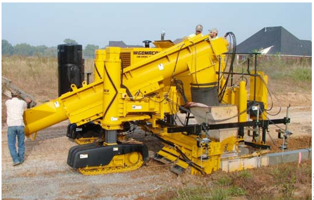
Their GT-3600 easily trims through grade with a 95 percent compaction requirement.
