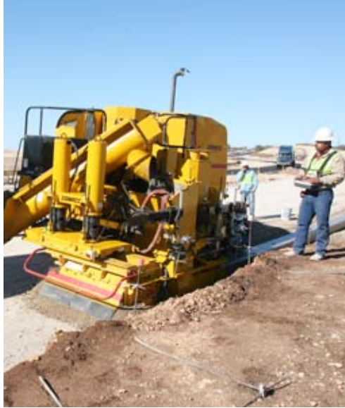
The GT-3400's can be ordered either right-side or left-side pour capable.
