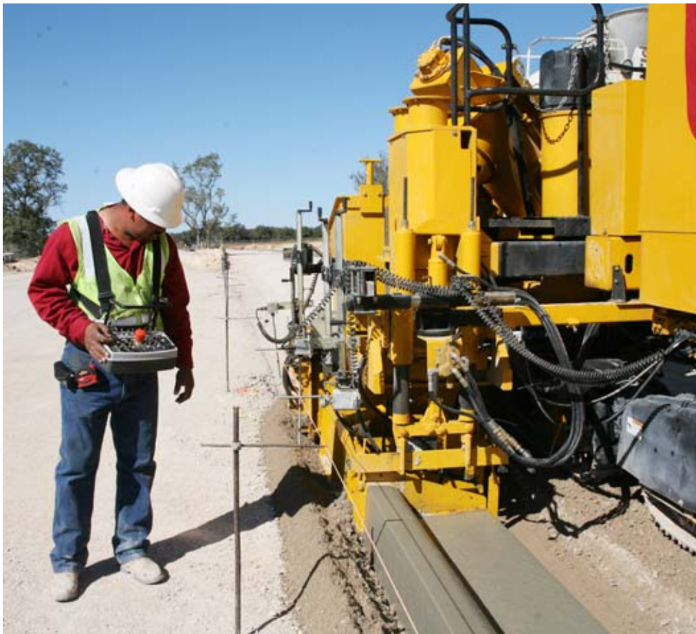
OMNEX Controls worked with GOMACO to develop the wireless remote for the new GT-3400, making it the first remote controlled curb and gutter machine.
