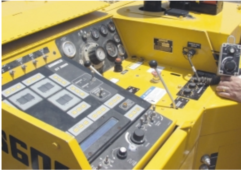
The G21 controller is operator friendly and a hand-held remote allows the operator to control travel speed and manual steer.
