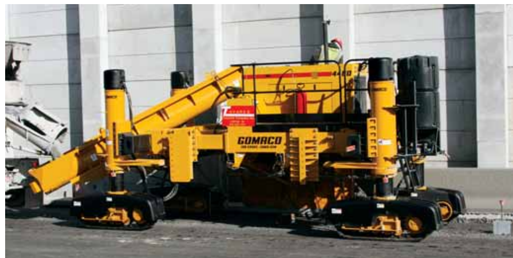
The new 4400 is a four-track barrier paver built for stability and symmetry to slipform right-side and left-side pour barrier and parapet walls.
