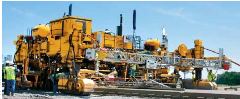
The four-track GHP-2800 with IDBI is paving 24 feet (7.3 m) wide, 11.5 inches (292 mm) thick. The IDBI is inserting 24 bars every 15 feet (4.6 m) on-the-go for the transverse joints.
