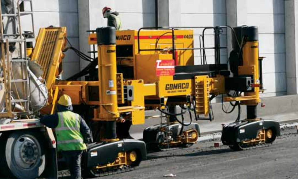
The new 4400 is a four-track barrier paver built for stability and symmetry to slipform right-side and left-side pour barrier and parapet walls.
