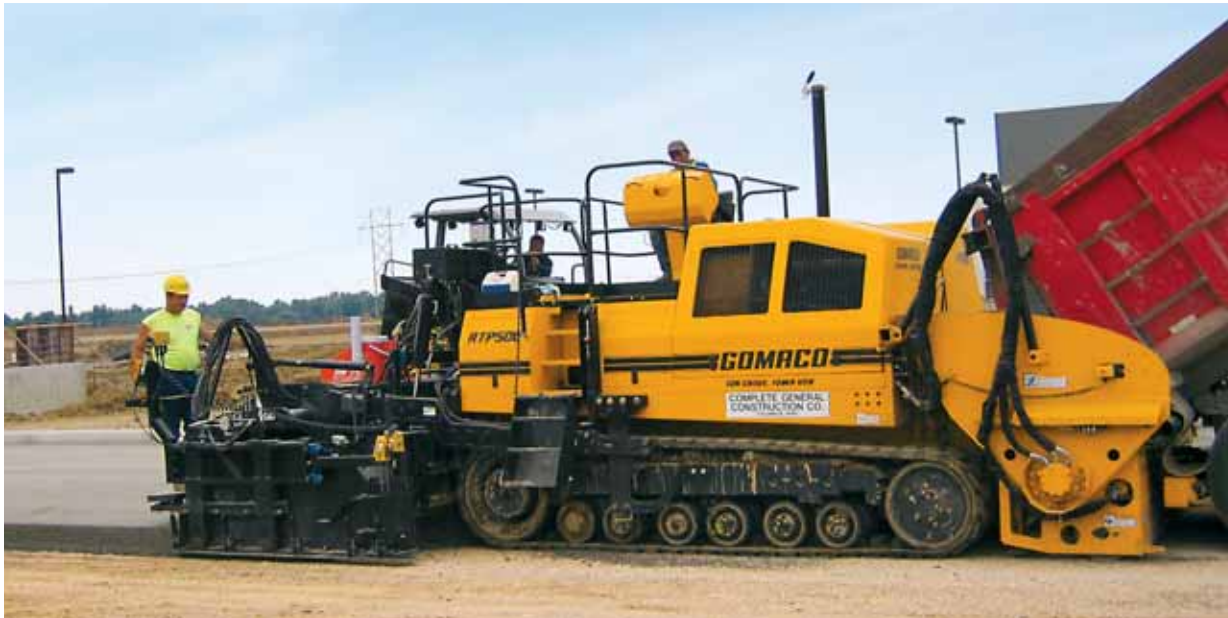
The GOMACO RTP-500 with RCC screed achieves density on a roller-compacted concrete project in New Albany, Ohio.
