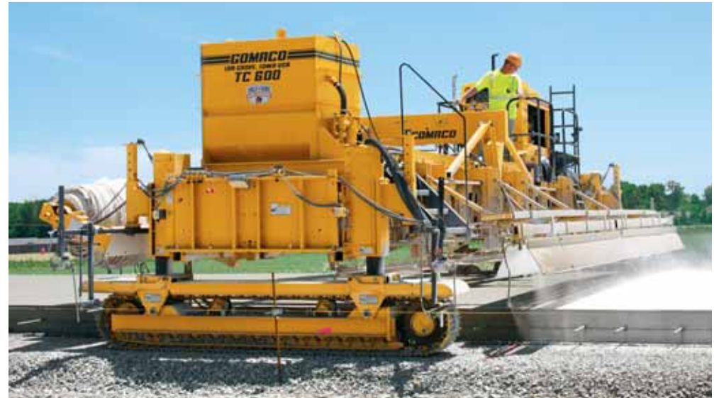
A new GOMACO T/C-600 texture/cure machine applies a longitudinal tine finish and white spray cure to the surface of new U.S. Route 24.
