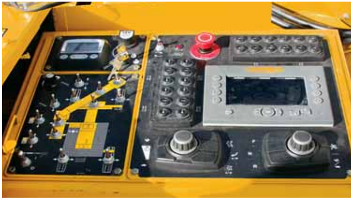
The 4400 features the GOMACO exclusive G+ control system, which slides for either right-side or left-side paving.
