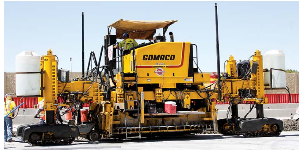
A 13 foot (4 m) paving mold remains mounted underneath the Commander III as it slipforms with its sidemounted mold. This allows for quick paving application changes.
