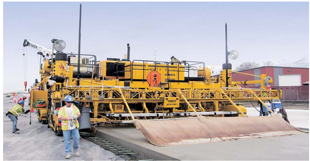
The GHP-2800 with IDBI attachment slipformed widths up to 26 feet (7.9 m) wide and paved a PI of zero for smooth concrete pavement on multiple paving sections.
