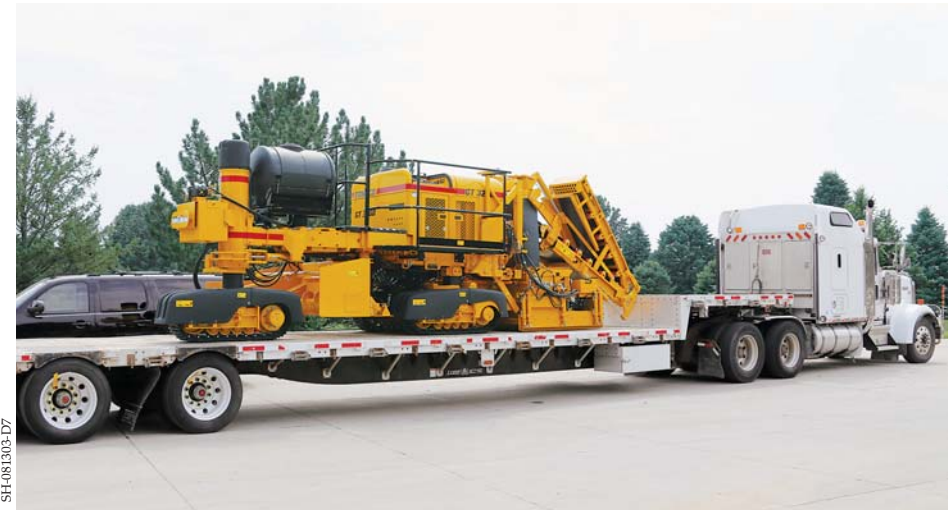
The GT-3200 sidewalk paver can be shipped fully assembled on one truck with the aggregate base mold or trimmerhead. The conveyor can be folded up for transport.
