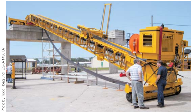
The RC Conveyor with telescoping tremie for placing the lean base material and concrete goes through final testing in Ida Grove, Iowa.
