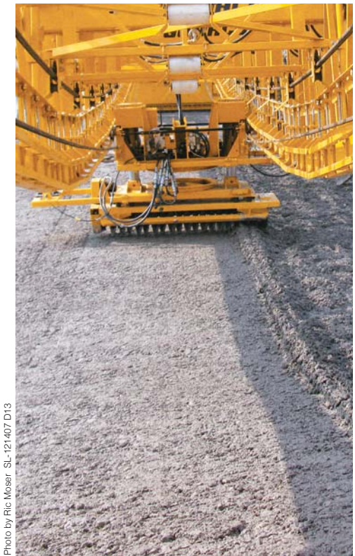
The SL-750's auger is 1524 millimeters (60 in) long and has a diameter of 248 millimeters (9.75 in).
