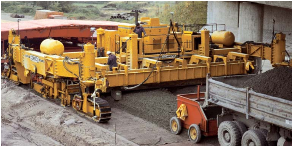
The GOMACO GP-5000, built in 1984, was the world's largest paver and had the ability to slipform 50 feet (15.2 m) wide. It was outfitted with a diverter plow and strike-off plate, two tie-bar inserters, and an automatic dowel bar placer for slipforming a project on the German Autobahn.
