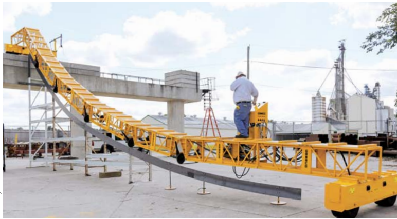
The GOMACO self-powered 4000 series Spanit work bridge is fitted with large turnbuckles that can be used to make manual slope adjustments.
