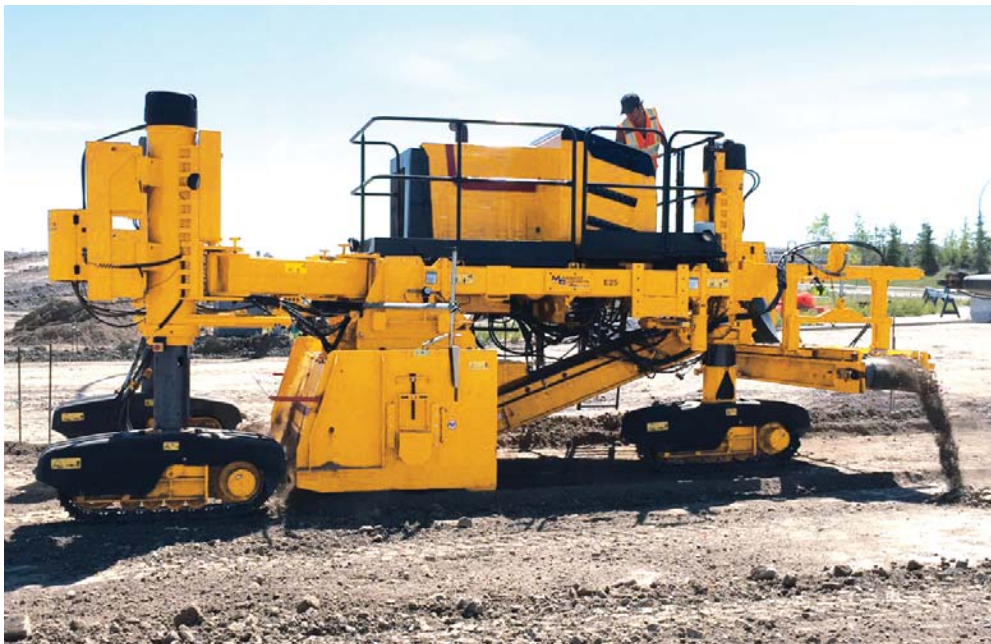
The Commander III trimmer has the ability to discharge the trimmed material to either side of the machine, either into the center of the roadway or over the stringline.
