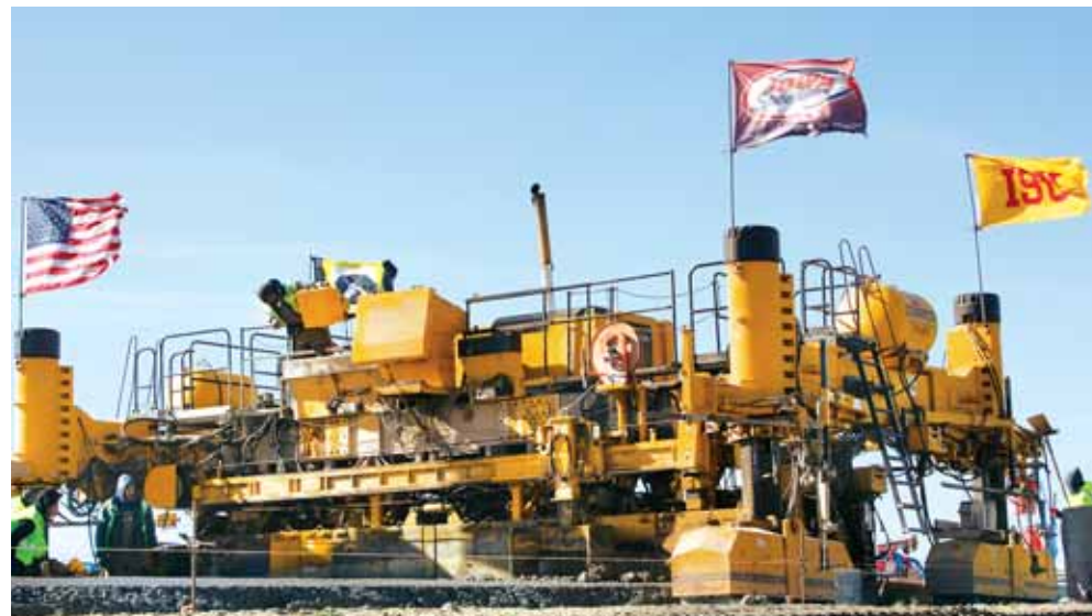
The GHP-2800 is equipped with the new GOMACO 5400 series mold that features a spreader plow mounted on the paver frame T-rail.
