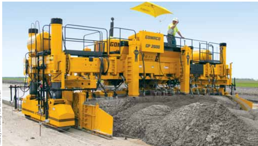
Opp Construction’s GOMACO RTP-500 rubber-tracked placer and two-track GP-2600 paver slipforms sugar beet pads.
