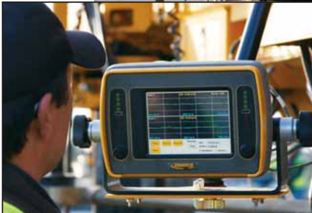
Two paver-mounted GOMACO GSI units monitor the smoothness in each driving lane. The information is instantly displayed and reviewed on a single touch-screen mounted on the side of the GHP-2800 paver.
