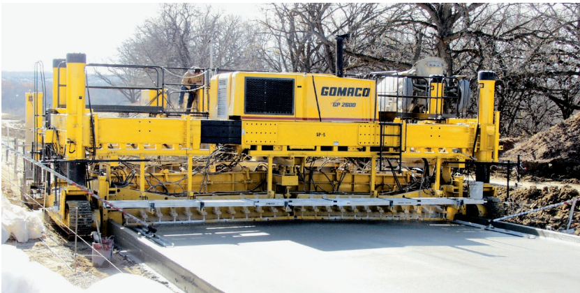
The GP-2600 has a modular telescoping frame that extends 6.5 feet (1.98 m) on the left side.
